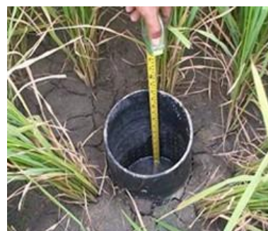
Water at 15 cm below the soil surface: Time to irrigate the field again
